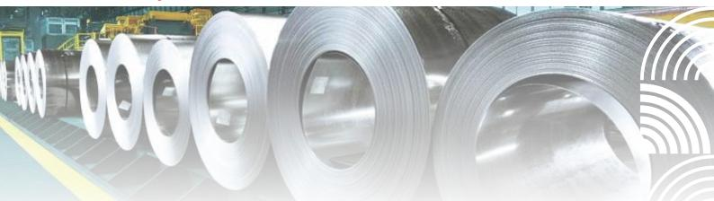
CR small steel products are thin and flat steel sheets that have undergone a process called cold rolling. This involves passing the steel through a set of rollers at room temperature, which compresses and elongates the material, resulting in a smoother and more uniform surface.
