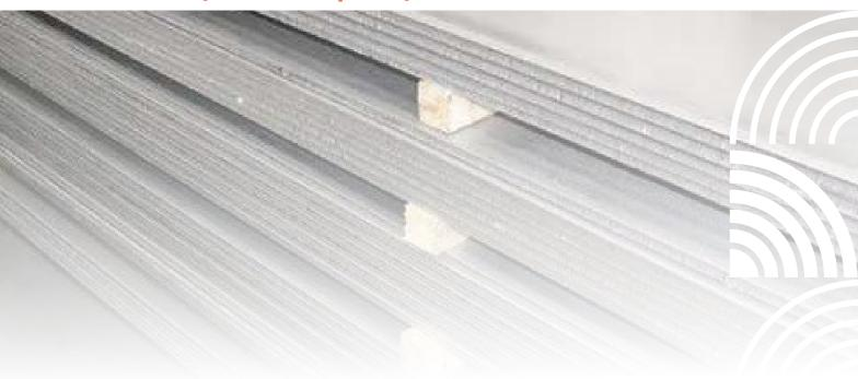
PMP plate, also known as Plate Mill plate, refers to steel plates produced through the plate mill process. These plates are manufactured by rolling and flattening steel slabs, resulting in large-sized plates with excellent thickness consistency and surface quality.
